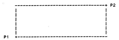
The scaling points P1,P2 have a different default depending on the plotter module, plus they may be manually set by controls on the plotter. Thus what makes sense to one plotter may be garbage to another.
