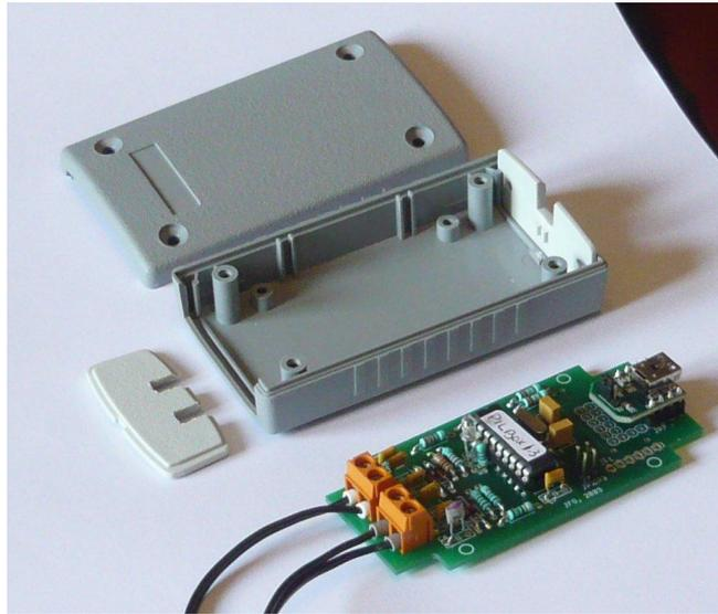
The top and bottom parts of the housing must be aligned, i.e. the 'notches' (the PILBox serial number is normally written on the top side 'notch') must be on the same side than the HPIL cable outputs.
